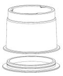
Step5:Remove sealing ring of chamber base.
